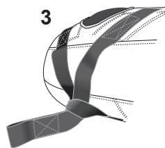
Special Note: The tow system should only be used as shown in this diagram. Towing from the top or bottom strap alone will cause the tube to function incorrectly and may risk damage to the cover or tube. Damaged caused by improper use will void your warranty.
